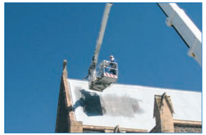
Cage rotation 90 degrees. Hydraulically extendable cage available as an option.
